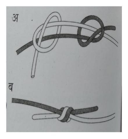
(To join two equal diameter ropes)
