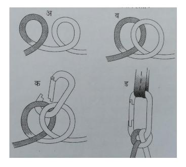
(To connect or attach rope to some anchor)
